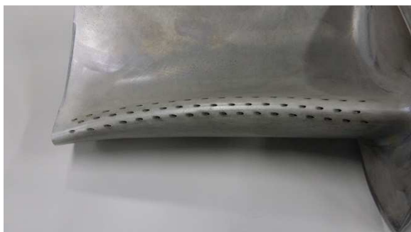
Figure 1: Hole patterns in a turbine blade
