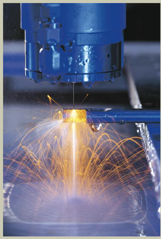
Figure 3. Laser MicroJet cutting is perfect for tool machining. It normally takes just a few minutes to cut a tool insert
