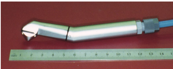
Fig. 5: Dental hand tool with water jet guided laser
