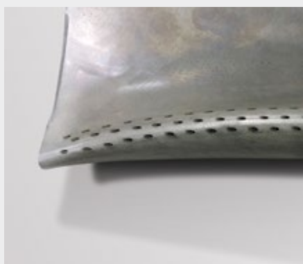
Energy & Aerospace: Drilling of turbine blades (superalloys + TBC)
